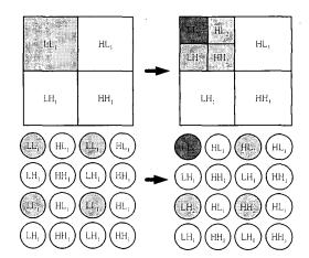
Fig. 8. Example of 2-level wavelet transform shows the in-place interleaving organization of wavelet coefficients, where a circle represents a pixel.
