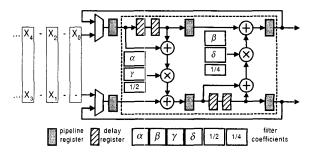
Fig. 4. Proposed folded architecture for 5/3 and 9/7 filter of DWT
