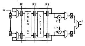
Fig. 5. Simplified block diagram with pre- and post- data formatter
