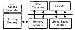
Fig. 9. JPEG 2000 system block diagram
